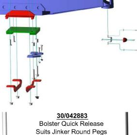
Suits Jinker Round Pegs High Tensile Capacity = 19,000kg
