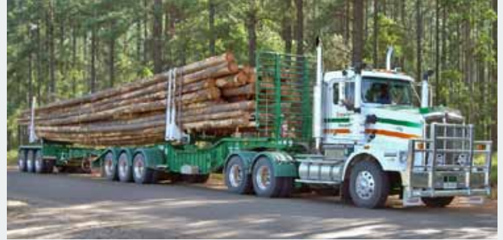
Triaxle-Triaxle — Long Load Mover. 19m single length loads on standard B-Double routes (26m)
