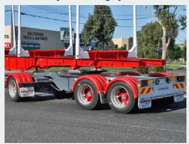
This unit can achieve a similar payload to a quad axle trailer with one less axle.
