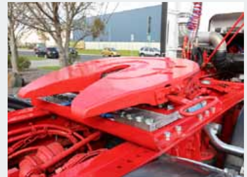
Extra Heavy option. 4x loadcells mounted under 5th wheel.
