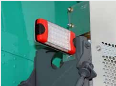
Limit light mounted on rear of prime mover.
