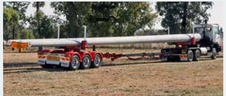
Triaxle Extendable Pole Trailer with multi-fit quick release bolsters to suit large beams or pipes.
