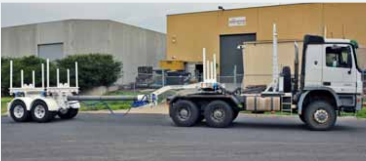
Tandem Pole Trailer with multi-telescopic extendable pole.
