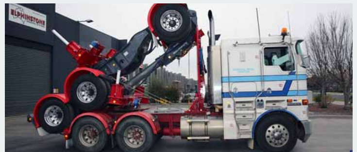
Easyster Pole Trailer Jinker with multi-fit quick release bolsters to suit large beams or pipes with the benefit of being able to load the trailer onto the rear of the truck for better traction
