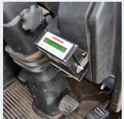
Easyweigh on-board scales with in-cab display
