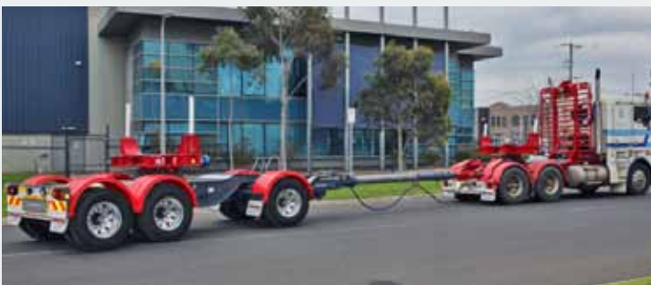
Easyster Pole Trailer Jinker with multi-fit quick release bolsters to suit large beams or pipes with the benefit of being able to load the trailer onto the rear of the truck for better traction
