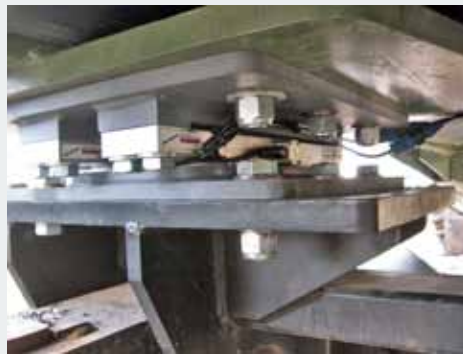
Suspension mounted loadcells
