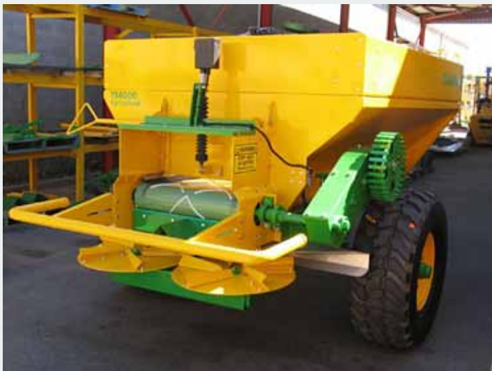
Trailing Spreader with loadcells mounted in the hitch pin and axle
