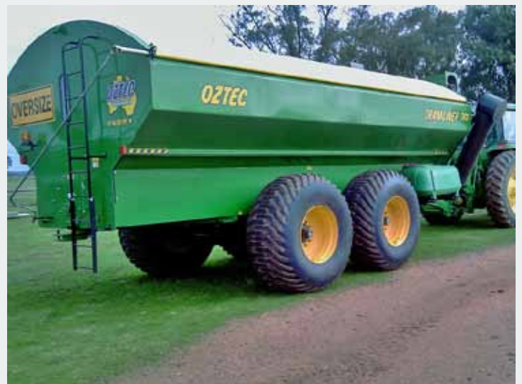
Large Trailer Spreader with loadcells at the draw bar and at the rear axles
