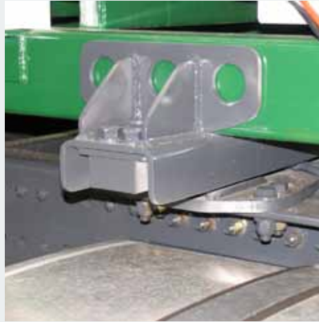
Loadcells fitted inside rigid truck chassis mount
