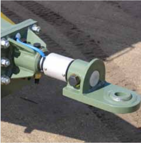
Loadcell drawbar mounting assembly suit trailing spreader
