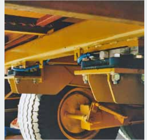
Loadcells mounted under trailing spreader axles
