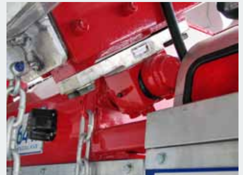
Loadcells mounted under pivot point
