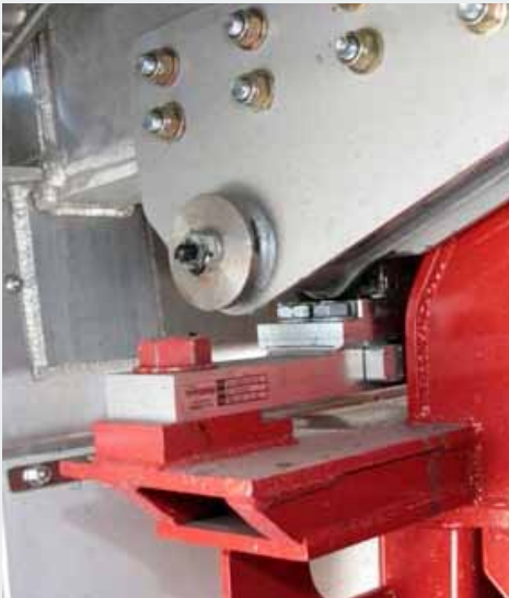
Loadcells mounted under pivot point
