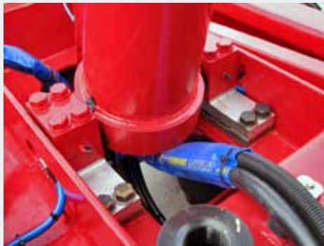
Loadcells mounted under hoist
