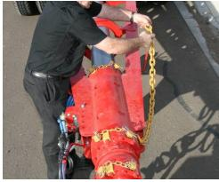
3. Use winch handle located on side of A Frame
