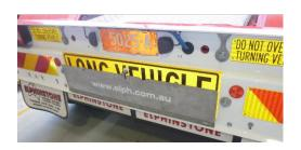
Fold **DOWN** LONG VEHICLE sign on rear of trailer when trailer is extended
