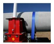
IF ONLY CARTING ONE POLE PLACE IN CENTRE AND STRAP DOWN WITH WINCHES ON DOLLY BOLSTERS (EXTENSIONS)
