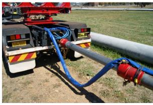
When at full length add in inter-connection cable and lash to pole
