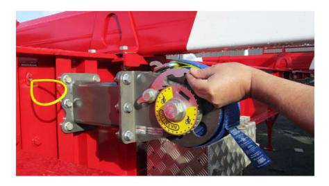
2. Unhook strap. This allows drum to run free and strap can be pulled off drum.
