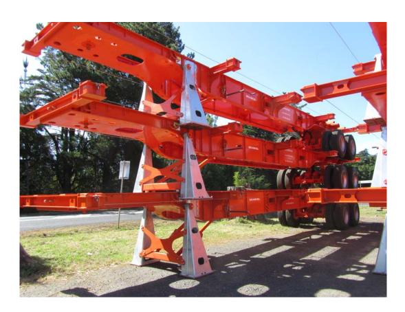
Ensure that landing leg is fully down and stays locked in over centre position on each trailer
