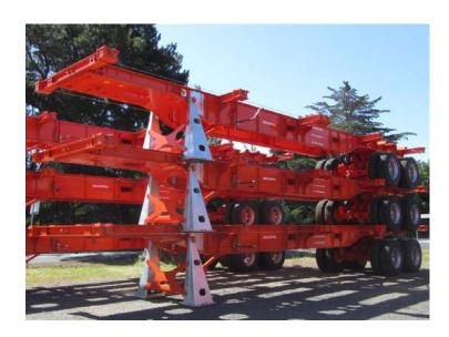
4. Ensure landing leg bump stops are sitting on top rails of bottom trailer and guides down sides of rails
