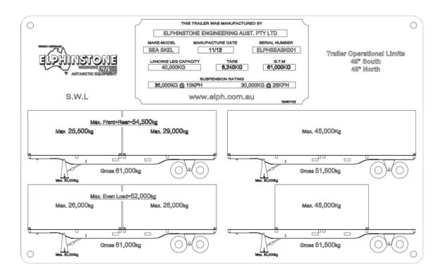
When loading two containers; the heaviest container should be at the rear.
